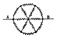
There are twelve resistors, arranged in a system as shown in the diagram, the value of each resistor being 1 ohm.
